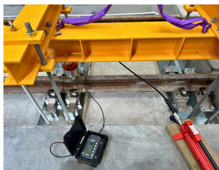
TRAKMATE test press is used for on-site calibration - no test train required
