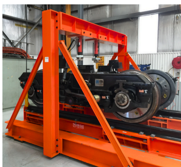
Bogie balancing press fitted with TRAKMATE loadcells
