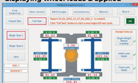
Touch screen PC controller displaying wheel loads & applied
