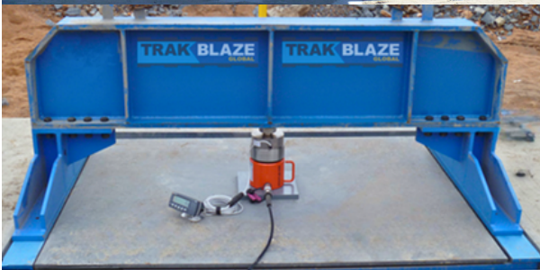
FORCE being tested and calibrated at site with a portable test press unit
